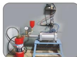
Pressure Cyclic Test
